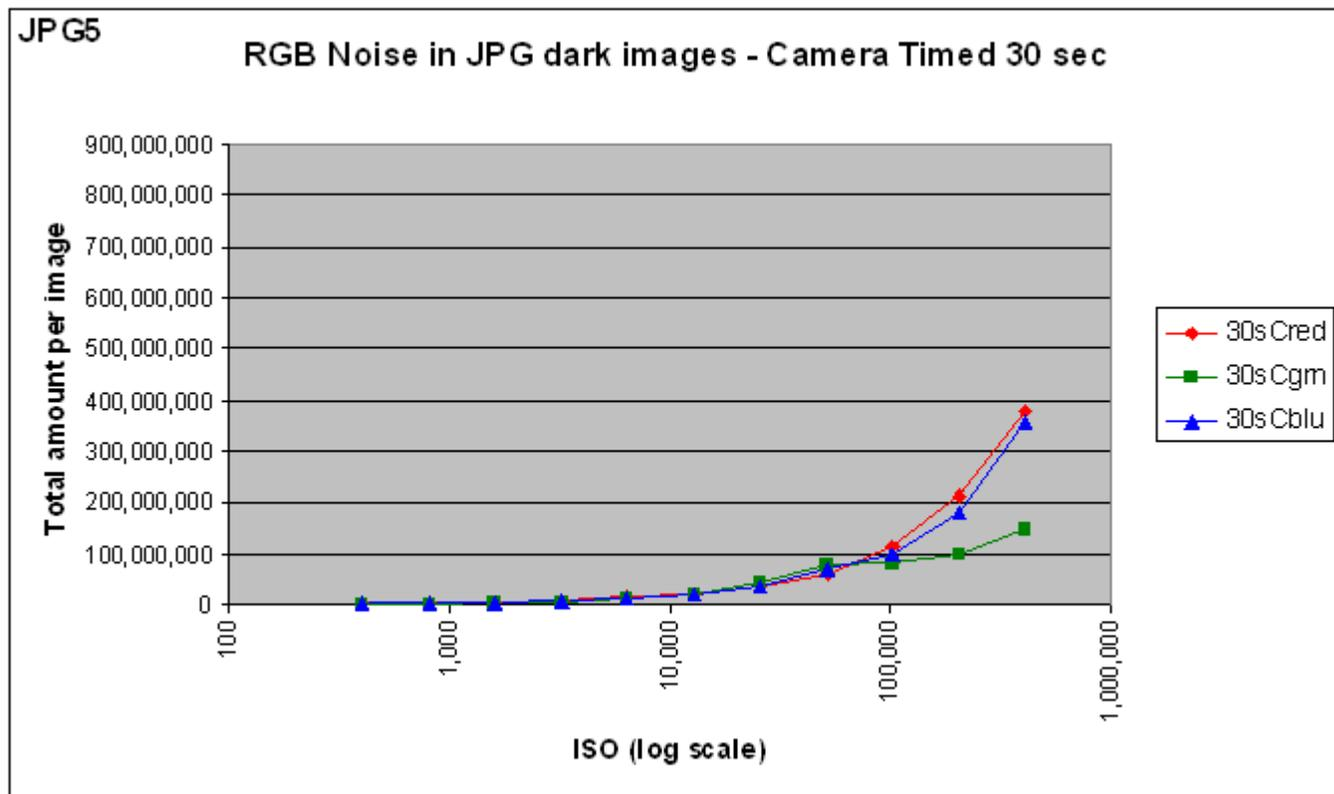
1. The individual JPEG R,G,B counts tracked together well up to ISO 51,200 after which the amount of "green noise" in the JPEG image is drastically altered (reduced) for both Camera-timed and BULB exposures.
